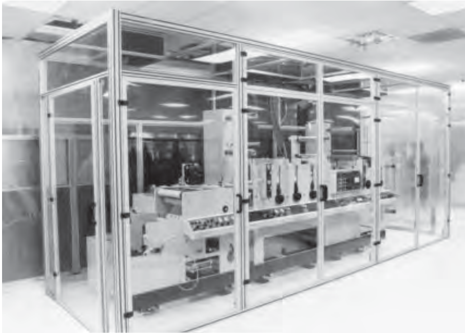
Machine safety enclosure using Lexan panels
